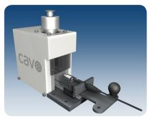
Ballard designed this Cavometrix semiautomatic crimp machine for creating Cavomate Series connectors.
