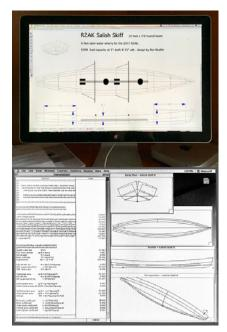
Using specialty hull design software, Mueller then exported a DXF file and brought it into Graphite to designate equipment placement and layout buildable lengths, nested together on 4'x8' sheets of plywood to be cut by his CNC machine.
